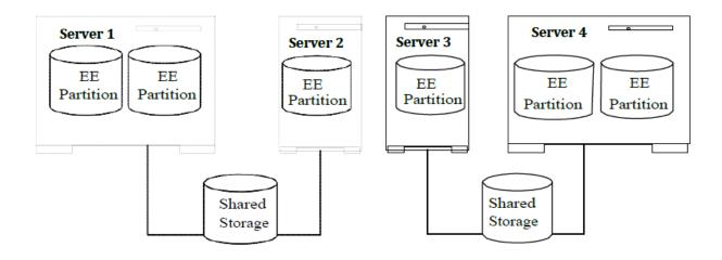
One DB2 instance with two database partition servers is protected on Server 1, one database partition server protected on Server 2, one database partition server protected on Server 3 and two database partition servers protected on Server 4. There is one LifeKeeper DB2 resource hierarchy on each server in the cluster. Upon failure, Server 1 and Server 2 assume each other's resources and Server 3 and Server 4 assume each other's resources.
