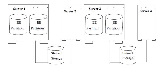
One DB2 instance with two database partition servers is protected on Server 1 and two database partition servers protected on Server 3. There is one LifeKeeper DB2 resource hierarchy on Server 1, extended to
