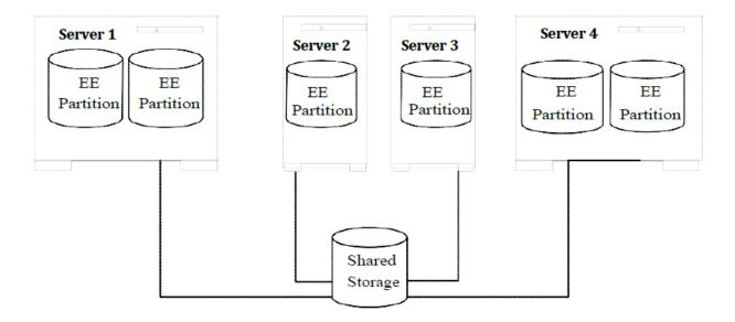
One DB2 instance with two database partition servers is protected on Server 1, one database partition server protected on Server 2, one database partition server protected on Server 3 and two database partition servers protected on Server 4. There is one LifeKeeper DB2 resource hierarchy on each server in the cluster. Each server in the cluster provides backup protection for the other in the event of failure.
