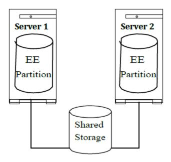
One DB2 instance with one database partition server is protected on Server 1 and one database partition server protected on Server 2. There is one LifeKeeper DB2 resource hierarchy on Server 1 and another DB2 resource hierarchy on Server 2. When a failure occurs each server will assume the other's resources.
