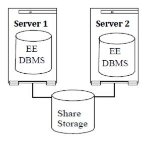
One DB2 instance is protected on Server 1 and another DB2 instance is protected on Server 2. Each server will assume the other's resources when a failure occurs.
