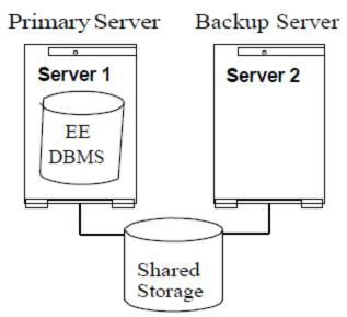
The DB2 instance is protected on Server 1. Server 2 will assume the DB2 resources when a failure occurs.
