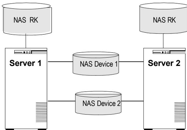
An active/active configuration consists of two or more systems actively running the NAS Recovery Kit software and importing file systems from NAS device(s).
