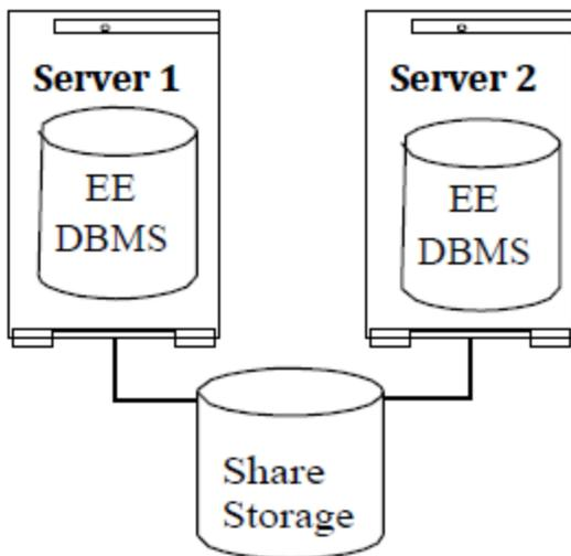
One DB2 instance is protected on Server 1 and another DB2 instance is protected on Server 2. Each server will assume the other's resources when a failure occurs.
