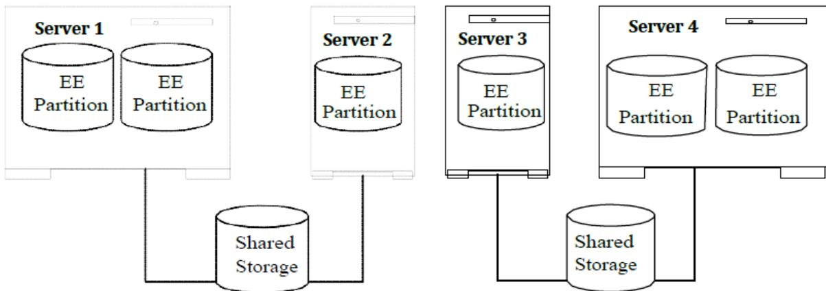
One DB2 instance with two database partition servers is protected on Server 1, one database partition server protected on Server 2, one database partition server protected on Server 3 and two database partition servers protected on Server 4. There is one LifeKeeper DB2 resource hierarchy on each server in the cluster. Upon failure, Server 1 and Server 2 assume each other's resources and Server 3 and Server 4 assume each other's resources.
