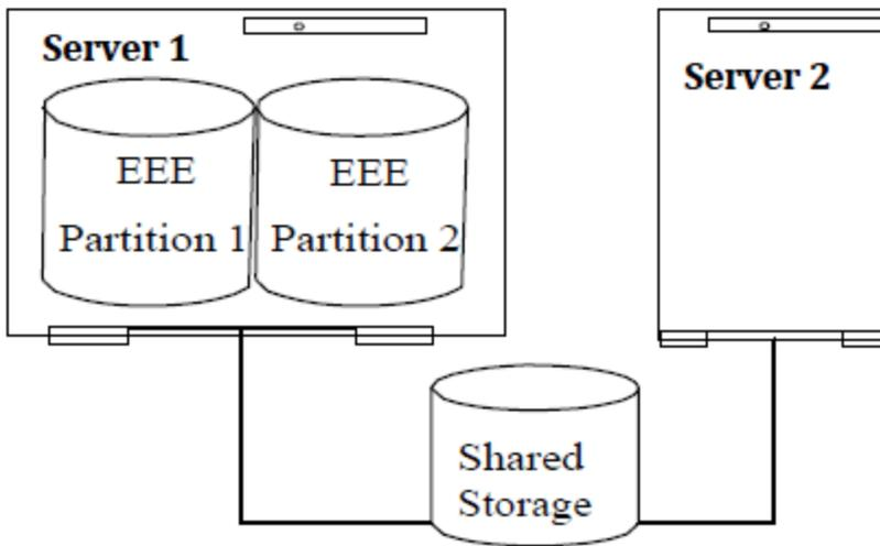
One DB2 instance with two database partition servers is protected on Server 1 with one LifeKeeper DB2 resource hierarchy. Server 2 will assume ownership of the DB2 resource hierarchy when a failure occurs.
