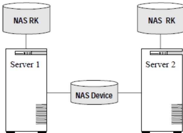
In this configuration, Server 1 is considered active because it is running the NAS Recovery Kit software and has imported (mounted) the file system from the NAS device. Server 2 does other processing. If Server 1 fails, Server 2 gains access to the file system and uses the LifeKeeper secondary hierarchy to make it available to clients.
