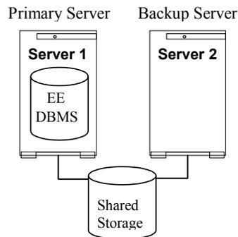
The DB2 instance is protected on Server 1. Server 2 will assume the DB2 resources when a failure occurs.
